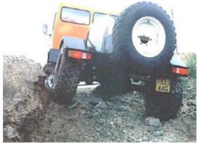
The RTT under test in a quarry whilst carrying a 1.5t payload. Traction and climbing ability in such adverse conditions is maintained due to the suspension systems ability to keep all four wheels firmly on the ground.
