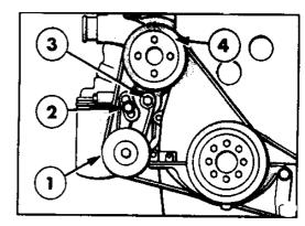
Fig. b1 - Water pump drive belt.
