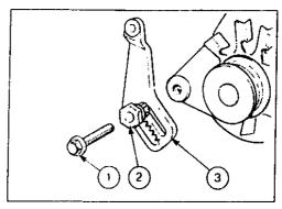
Fig. a2 - Rack & pinion adjuster.
