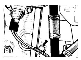
Cylinder block drain bung.
