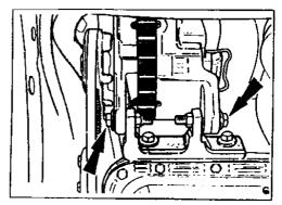
Fig. a1 - Alternator mounting bolts.
