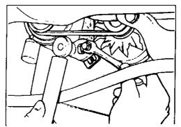
Fig. a3 - Tensioning method for alternator drive belt.
