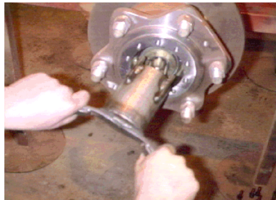
Tightening nut with special tool
