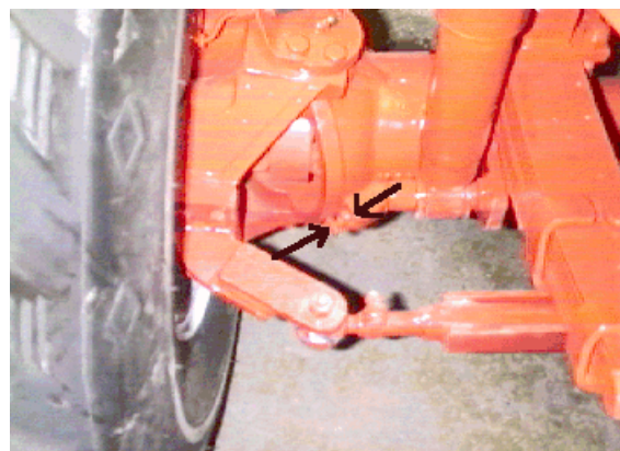
Steering stop adjustment
