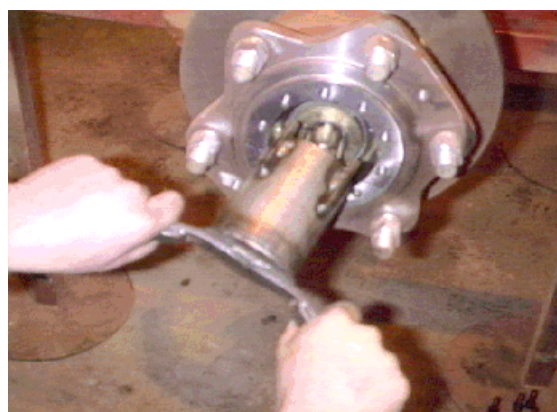
Tightening nut with special tool
